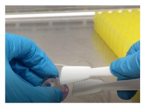
4. Add media to test chamber. Media should passively diffuse into the devices when opened. You may also add media to devices; we recommend not to exceed 600 ul. Media line should be above the chamber openings.
